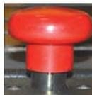
Use the E-stop as a service brake to secure the stacker when parked.
