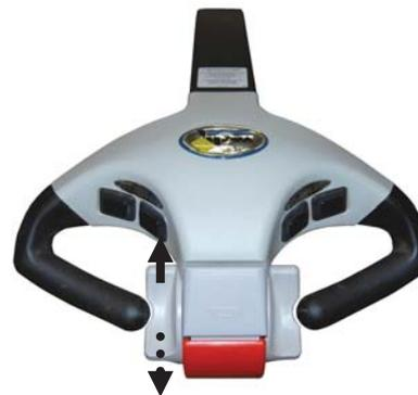
The degree of rotation determines the speed of movement, so the farther you press the wheel in either direction, the faster the stacker will travel, up to a maximum speed of ~3mph when unloaded or ~2.6mph when loaded to capacity. Simply by releasing the movement control, the stacker will decelerate to a complete stop.
