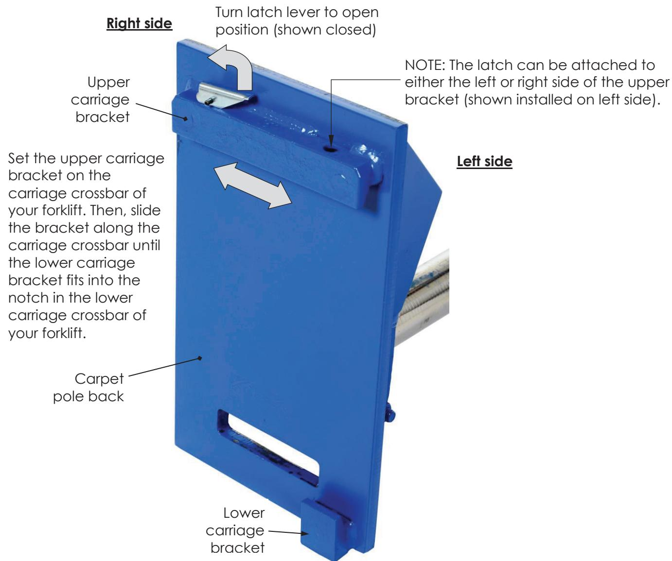
**Step 3:** Slide the upper carriage bracket along the carriage crossbar. Adjust position to allow the lower carriage bracket to fit into the notch in the lower carriage crossbar (of the forklift). The notch is probably located at the center of the crossbar. Next, slide the back plate to the left or right as necessary to center the carpet pole on the carriage.
