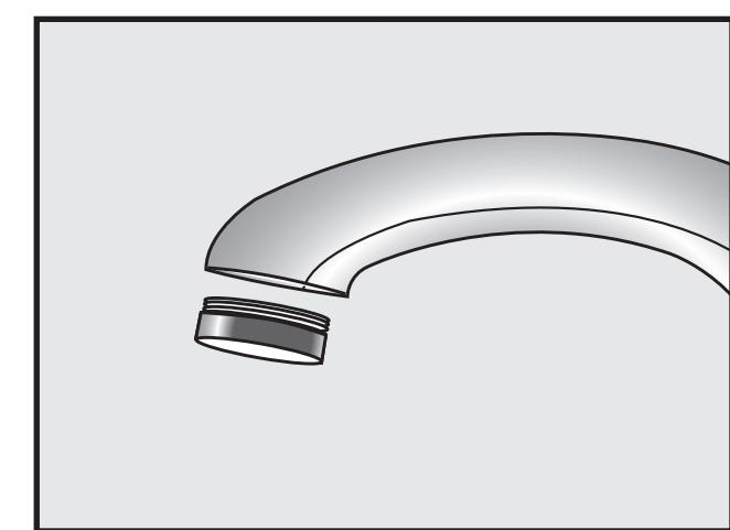
Aerators are available in additional sizes (1.5 gpm & 2.0 gpm) for purchase, if you desire to increase water flow. To install the new aerator, remove the existing aerator by hand. If the aerator is too tight to be removed by hand, it is recommended that a strap wrench be used to loosen it. Once the old aerator has been removed, the new aerator can be installed and hand-tightened in its place.
