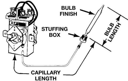
\* Replacement controls with "Nickel" referenced in ordering chart will be nickel plated for the first 30" of the diastat. EXAMPLE: Control with 36" capillary and 10" bulb = 16" of capillary will be non-plated.
