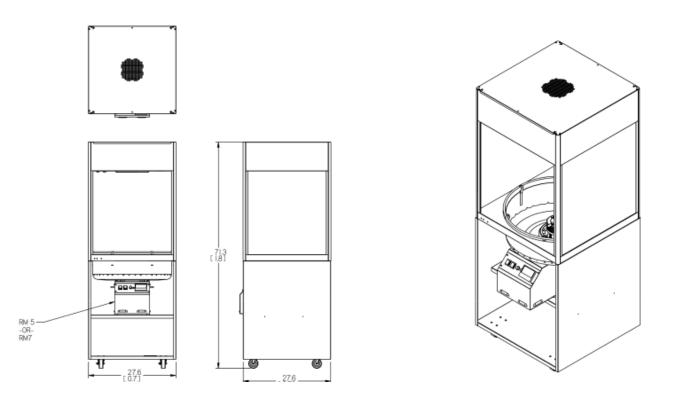
If equipped with optional Cretors Cotton Candy/Floss Stand, the Ringmaster body should be installed into the stand without the bowl on. Drop the feet of the RM body into the embossed dimples in the shelf. Plug the RM into the outlet located in the back of the Floss stand. Now install the bowl into the cabinet on top of the top shelf in the floss stand.
