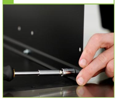
Before connecting the last two bolts at the bottom insert the extension leg. Using a ½" bolt, connect the extension leg, the side panel, and the back panel together. The foot of the extension leg should face downwards.
