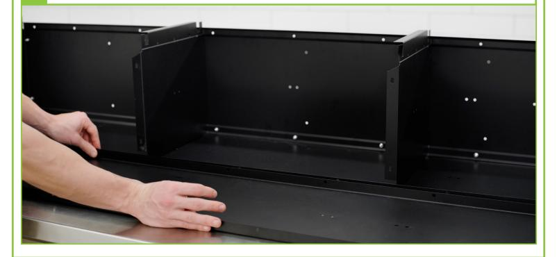
Use ½" bolt to connect the second back panel and the second side panel to the first back panel. The bolt should connect all three components.
