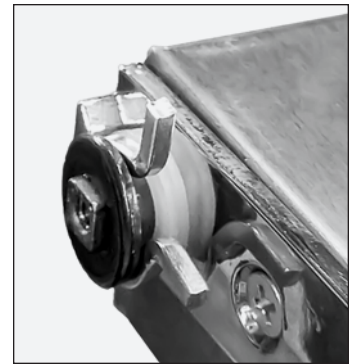
Fig. 7. Keep the washers in their original order.
