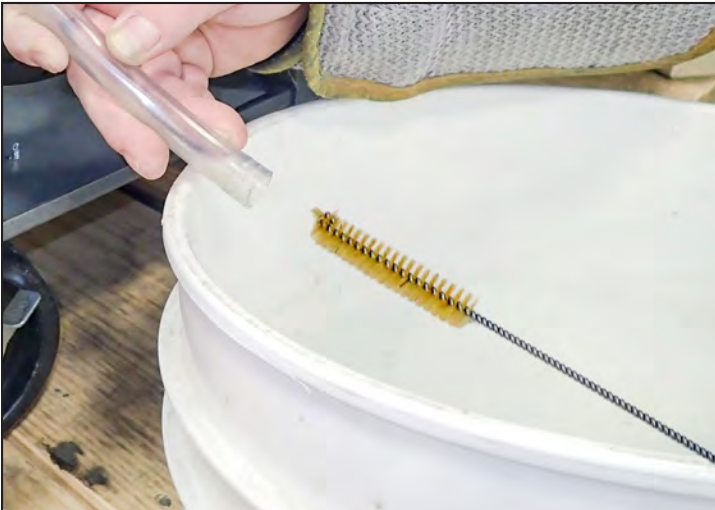
Fig. 2. Catch trapped liquid in a large container.
