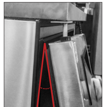
Fig. 10. If needed, only use shallow angles when positioning the door.
