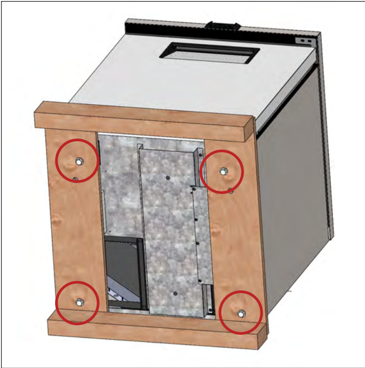
Fig. 3. Remove all shipping bolts.
