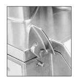
4) Position the head of the vegetable preparation machine on the motor shaft. The fastening hook should now be facing you, on your right.
