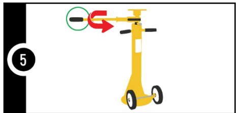
Step 5: Use handle in counter-clockwise motion to lift to desired height.
