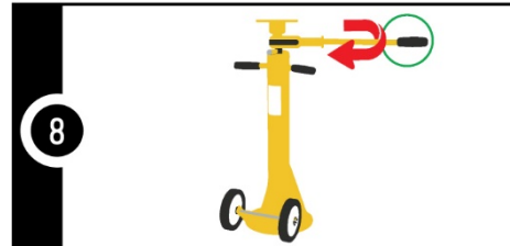
Step 8: Use handle in clockwise motion to lower to desired height.
