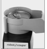
4) Place the cutting plate of your choice onto the discharge plate. It may be necessary to rotate the plate until it drops fully onto the discharge plate.
