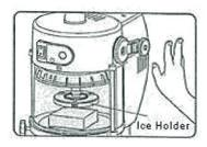
2) Confirm that the ice holder does not descend when a supporting hand is removed from the crank handle.
