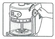
5) Turn the crank handle counter-clockwise to keep the ice holder to the lowest level. Close the sliding cover(shaving shield). This is for safety reasons.
