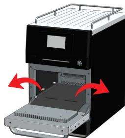
**3- FULLY OPEN THE EASY CLEAN LINER FLAPS, ADJUSTING IT UNTIL IT IS PROPERLY SEATED.**
