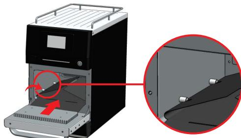
**2- FOLD SIZE FLAPS AND FIT THE EASY CLEAN LINER INTO THE EQUIPMENT AND THEN SIDE GUIDES AS SHOWN.**
