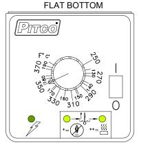
This control was developed by Pitco to replace bulb and capillary thermostats in fryer applications. It utilizes the latest in microprocessor technology and allows a host of features not practical with a simple capillary t-stat. Features include a selectable start up melt cycle, drain valve interlock, faulty probe detection, and a boil out mode.
