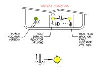
HFB indicator flashes 7 times, pauses, then repeats, until the drain valve is closed
