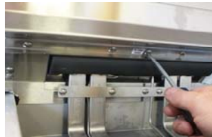
Picture 1 Use a flat screw driver to remove the screw marked "Reset Button"(Full pot shown). SELV14T reset buttons are under the outer Screws.
