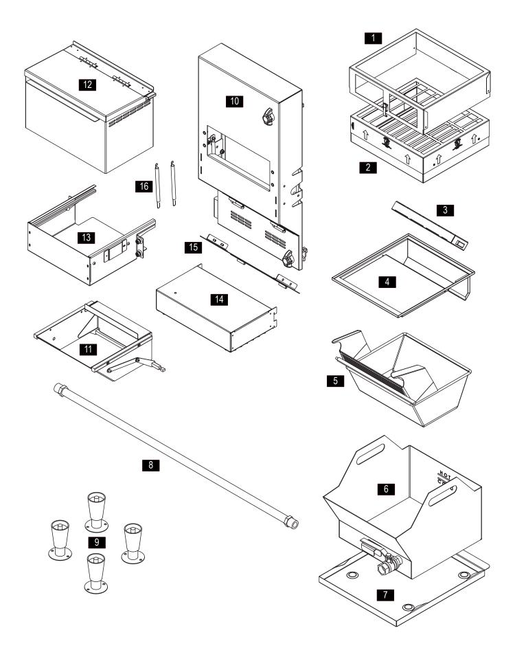
6. Tilt Perfect Fry unit to one side and install 2 adjustable legs, repeat process for other side.
