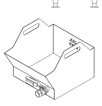
8. Pour frying oil into vat. Fill to **COLD** level mark. Use commercial grade deep fryer cooking oil. DO NOT OVERFILL
