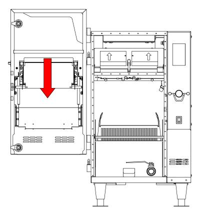
10. Install front panel using lift off hinges and close front panel. Rotate latches 180° clockwise to secure in place..
