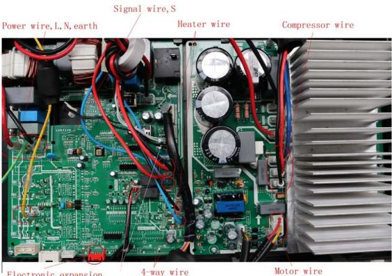
Electronic expansion 4-way wire valve T3, T4, T5 temperature sensor
