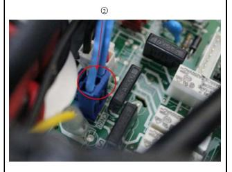
3) Pull out connectors of the compressor top temp. sensor, condenser coil temp. sensor(T3),outdoor ambient temp. sensor(T4) and discharge temp. sensor(T5).
