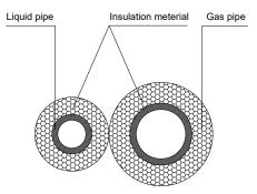
> The insulation material at the joint pipe shall be  $5\sim10$ cm longer than the gap of the insulation material.
