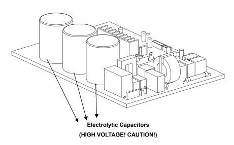
For other models, please connect discharge resistance (approx.100 $\Omega$  40W) or soldering iron (plug) between +, - terminals of the electrolytic capacitor on the contrary side of the outdoor PCB.
