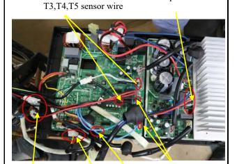
Electric pipe heater and Crankcase electric E Heater wire Motor wire 4 way valve
