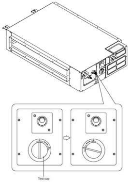
2.2 Power on and let the air conditioner operate for cooling. Check operation status of drainage pump, and then connect the plug of water level switch, check the operation sound of water pump and observe whether the water can discharge through the transparent hard pipe at drainage outlet. (In light of the length of drainage pipe, water shall be discharged about 1 minute delayed)
