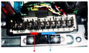
Remote on-off ports Central control ports
