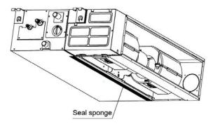
③ When install the filter mesh, please plug it into flange inclined from air return opening, and then push up.
