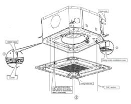
Tighten the screws under the panel hooks till the panel closely stick on the ceiling to avoid condensate water.
