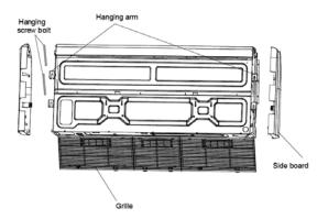
Locate the hanging arm on the hanging screw bolt. Prepare the mounting bolts on the unit.
