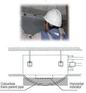
Adjust the position to ensure the gaps between the body and the four sides of ceiling are even. The body's lower part should sink into the ceiling for 10~12 mm. In general, L is half of the screw length of the installation hook.
