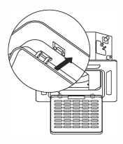
Connect the 2 wires of the decoration panel to the mainboard of the unit.
