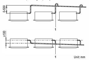
T-joint converging drain pipes
