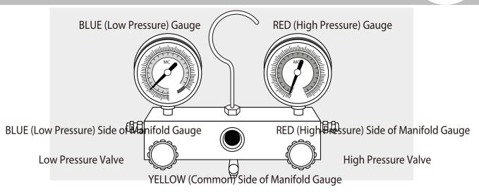
Caution: Systems are precharged with refrigerant (entire amount necessary for the system set has been charged into the outdoor section). The line sets and the indoor units are not charged, and must be evacuated prior to releasing the refrigerant from the outdoor unit to the rest of the system.
