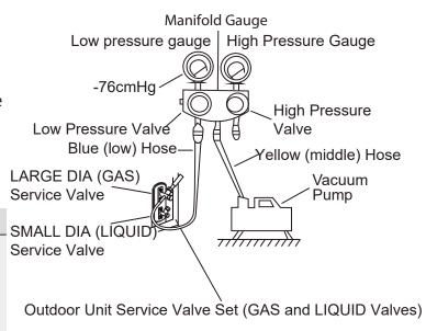
1. Connect the blue (low side) hose of the manifold gauge to the service port on the outdoor unit's GAS SIDE valve (use a 1/4" to 5/16" port adapter if
