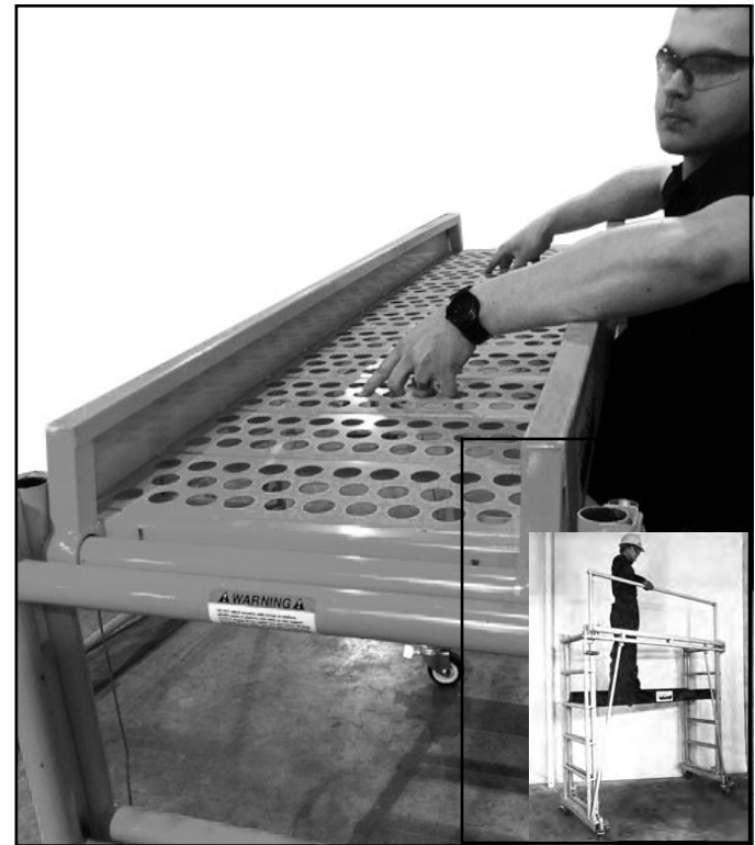
8) For platform heights from 2' to 6'10", the deck may be placed on lower rungs. For added safety use guard rails even when deck is on lower rungs.
