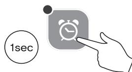
4. To CANCEL timing, press and hold 'Off Timer' button for 1 second. It will then switch the timer off automatically.
