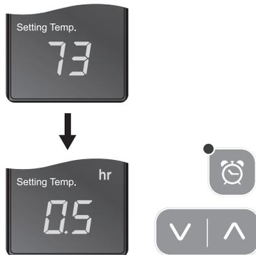
1. When unit is operating, press the 'Off Timer' button and set the length of time you want by pressing  $\wedge$  or  $\vee$ . Each time you press the button you will increase the 'time to off' period by 30mins. up to 10 hours, and 1 hour up to 24 hours. The display will show 0.5 for 30min and 1 for an hour. One and a half hours will show 1.5.
