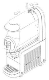
2. Push the lever upwards and then remove the bowl.
