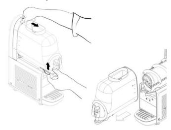
3. Remove the auger by sliding it off of the evaporator cylinder. Then remove the outer magnet rotor assembly.
