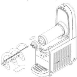
6. Replace the bowl by pushing it towards the back wall, making sure it fits properly onto the gasket. The locking lever will be lowered until it rests on the drip tray surface.
