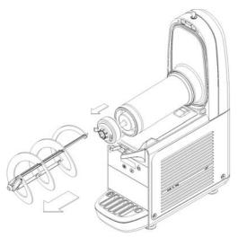
4. Remove the gasket from its housing.
