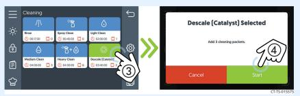
The oven heats to the required temperature for the descale catalyst cleaning cycle, then the cycle starts.
