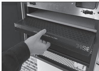
1 Removing the Activated carbon filter
