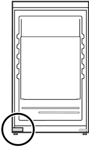
12. Screw the hinge angle and fix covers.
