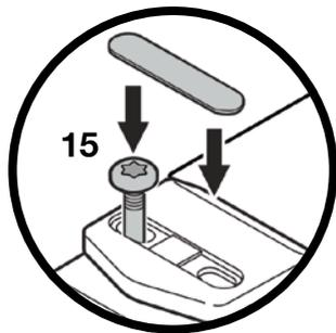
15. Insert bearing bolts. Align the door sideways and tighten the bearing bolts.
