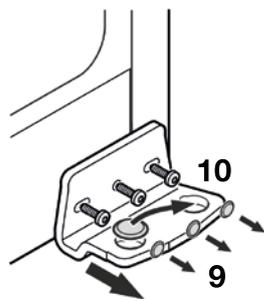
11. Remove the cover plate, turn it by 180° and reinsert it on the opposite side.
