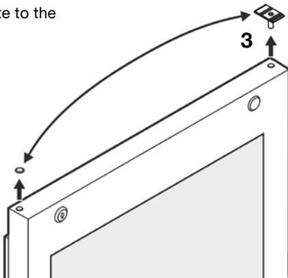
4. Adjust the lock and cover plates in the door to the other side.
