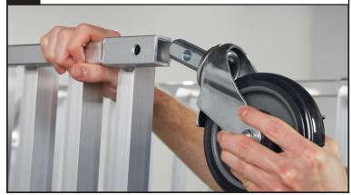
Once the casters are properly aligned, the remaining (2) Short Crossbars can be installed on the bottom of the rack using the 14mm Bolts.\*\*\*
