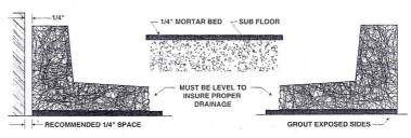
NOTE: Mortar should cover the entire area between receptor and building floor. (1/4" min.)
