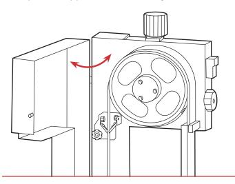
**2.** Loosen the tension knob at the top to take the blade off the wheels.
