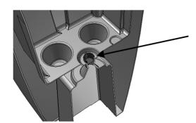
For indoor use, press the red plug down firmly into the overflow drainage hole to seal the planter before use.
