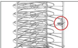
1. Insert the core temperature probe into the white ceramic tube on the mobile plate rack.
