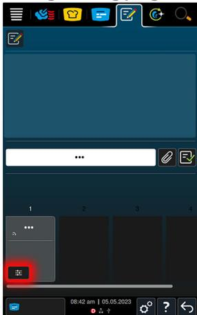
After selecting a cleaning program, press
