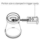
**INSTALL CLOSER PLATE** into unit body.
