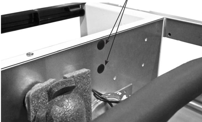
3. Assemble bracket to left-hand top rail with three provided screws.
