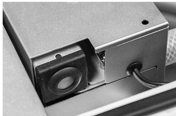
8. Attach connector to bulb.
