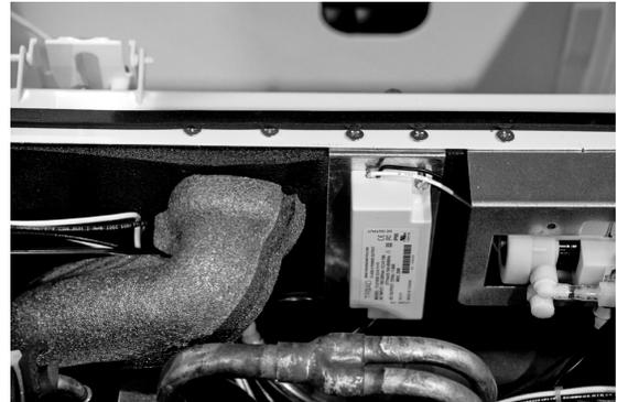
**Step 2** Route line voltage wires (black & white) through line voltage Heyco fitting. Disconnect L1 & N wires and install L1 & N of wiring adapter to the incoming power supply wires. Connect removed wires and LuminIce® wires to adapter.
