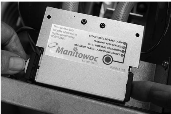
5. Remove retainer from old bulb and install on replacement bulb.
