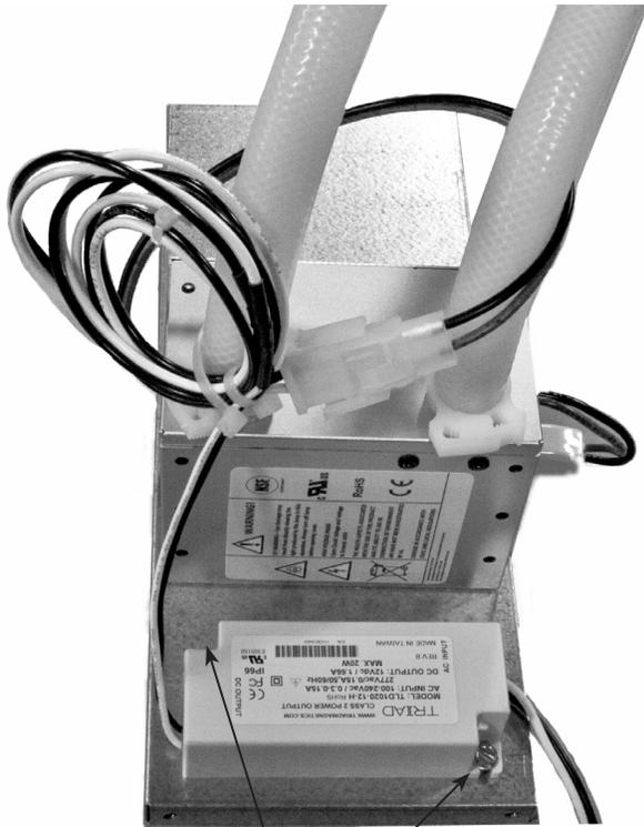
Mount LuminIce® And Power Supply To Bracket
