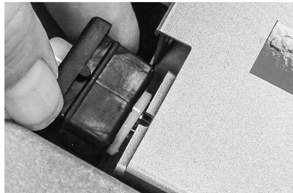
7. Insert bulb until it seats in the retainer stop on the opposite end.
