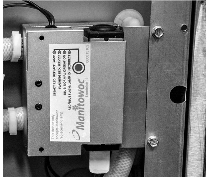
6. Mount power supply on the left side with two screws.
