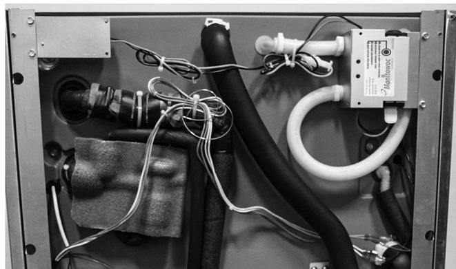
8. Reinstall bin, wire connectors and all panels, then test run. A noticeable draft will be emitted from the upper hose adapter during operation.
