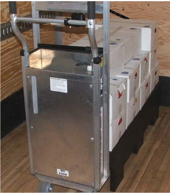
Figure 1: CooLift secured under a loaded pallet with the holding brake engaged
