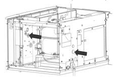
8. Connect the probe molex connector into the bin level port on the control board as shown.
