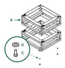
**2.** Adjust each foot (B) to the desired height. Ensure the height of the nut results in a level frame.
