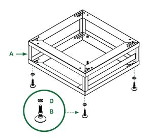
**4.** Place the stand on its feet to ensure that it is stable and level.
