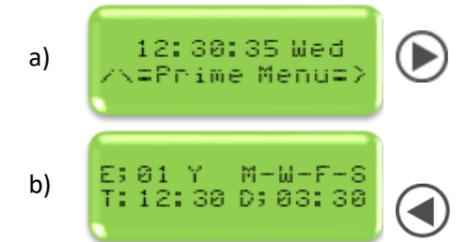
**Step 2:** (a) Adjust the access code by select Y or N to keep current code (b) Press right to access the time and date settings. Adjust accordingly and press right to get back to the main menu.
