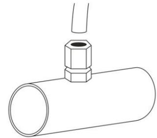
**Step 3:** Now connect the delivery tubing to the Pipe Injector, turning the compression nut clockwise until hand tight.
