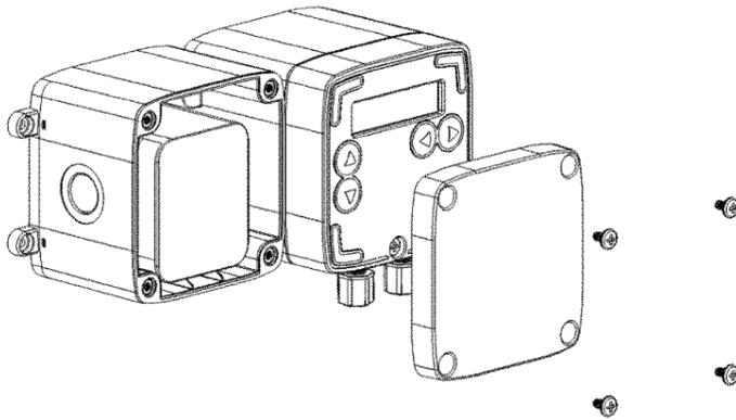
**Step 2:** Replace the x4 D Cell batteries with a high quality alkaline batteries for optimum performance and longevity. Now replace the battery holder in its enclosure and re-secure the lid.
