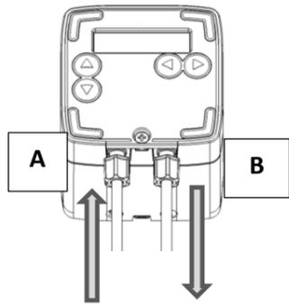
**Step 1:** Ensure there is no power to the unit; connect the suction tube from the chemical container to **(A)**. Now connect the delivery tube from **(B)** to the drain or injection point.
