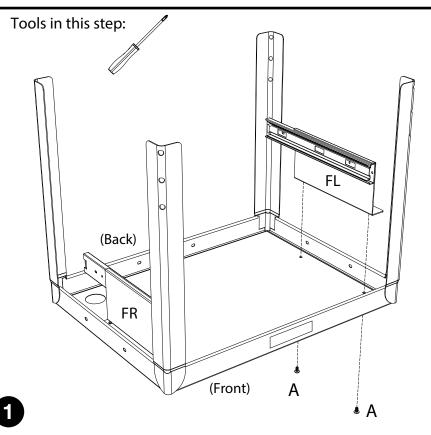
Take top shelf of metal cart and lay on side. Collect parts: FL, FR and A. Align brackets with screw holes on top of shelf. Insert screw A and tighten with screwdriver. Do not fully tighten until shelf is attached.
