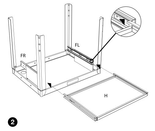
Collect part: H. Align the pullout shelf H runner so that the runner snaps into place into the FL & FR brackets. Pull the shelf out to make sure it is fully seated. Tighten screws A. Pullout keyboard shelf assembly is now complete.
