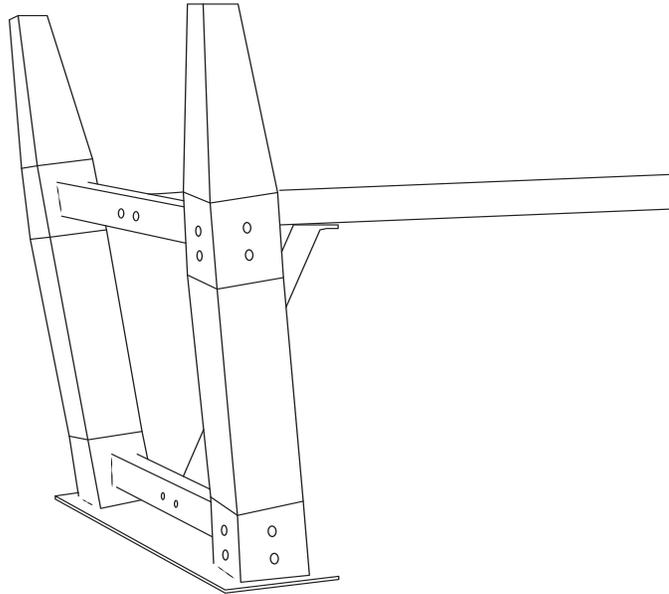
**7** Secure Iron Side Bottom Braces (Part B) to Connector Bar (Part D) using Button Nut ③ from the outside and Button nut screw cap ⑤ from the opposite side using both Allen Wrenches simultaneously. Repeat for other side.
