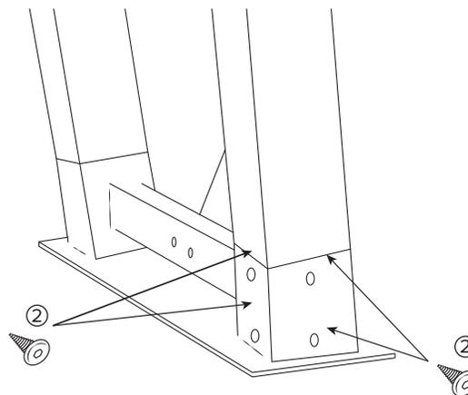
**10** Place and secure Adjustable Footpad ① to bottom of the Table Base Legs (Part A).
