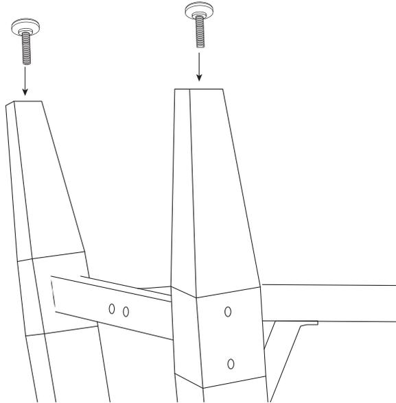
**11** Next, turn base right side up. Secure legs to Iron Side Top Brace (Part C) using Round Cap Wire Screws ②.
