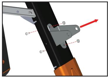
2B. Using a 1/8" allen wrench and 3/8" wrench remove and discard the bracket, screws, and lock nuts.
