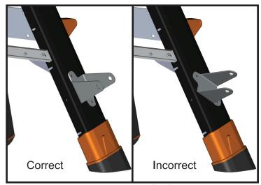
3. Determine correct bracket for front and back. Sides of bracket should be parallel with fiberglass rail.
