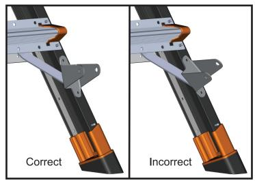
3. Determine correct bracket for left and right. Sides of bracket should be perpendicular to bottom rung.
