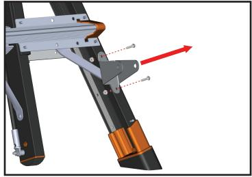
2. Using a 1/8" allen wrench and 3/8" wrench remove and discard the bracket, screws and lock nuts.
