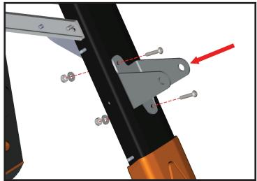
4. Line up the new bracket, then attach and tighten the new hardware as shown with a 1/8" allen wrench and 3/8" wrench.
