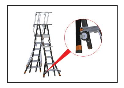
TIP & GLIDE™ WHEEL REPLACEMENT (SKIP TO PAGE THREE FOR SIDE TIP WHEELS)
