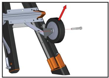
1. Using (2) 9/16" wrenches loosen and discard the wheel, bolt, and lock nut.
