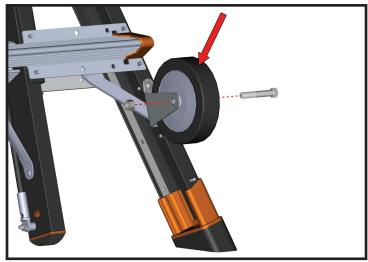
5. Align new wheel with bracket, then using (2) 9/16" wrenches, tighten the nut and bolt.
