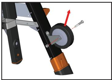
1B. (If replacing side tip wheels) Using (2) 9/16" wrenches loosen and discard the wheel, bolt, and lock nut.
