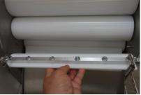
The #1 scraper lays under the middle roll and attaches to the scraper pins on the inside walls of the machine. The beveled edge points in between the middle and bottom roll.
