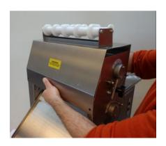
Remove the safety cover by removing the four thumb screws.
