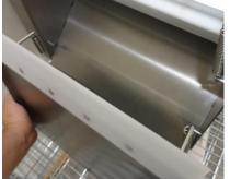
The #2 scraper lays on top of the bottom roll and is attached to the discharge tray as one piece. To remove the tray reach under the discharge tray and detach the scraper springs from the pins. Lift the tray up towards the machine and scraper will dislodge from the scraper pins.
