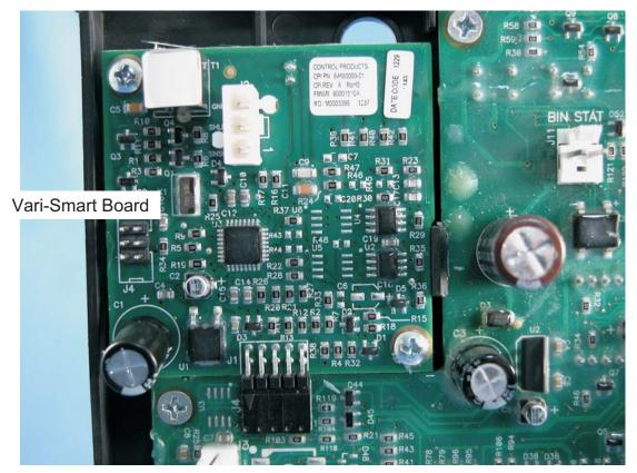
**Installing Vari-Smart Board**
