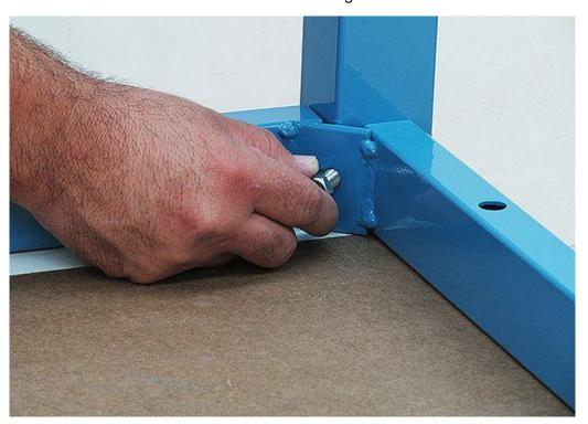
**4.** Tighten until lock washer is flat. It doesn't have to be tighter than that.
