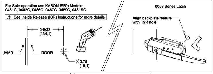
Ø 1/4 (6mm) Mounting fasteners not provided
