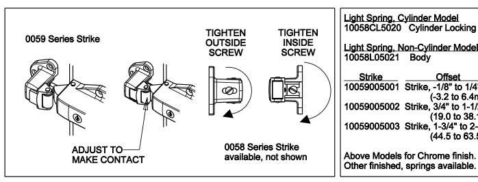
10058CL5020 Cylinder Locking Body Light Spring, Non-Cylinder Model 10058L05021 Body Strike **Offset** 10059005001 Strike, -1/8" to 1/4" (-3.2 to 6.4mm) 10059005002 Strike, 3/4" to 1-1/2" (19.0 to 38.1mm) 10059005003 Strike, 1-3/4" to 2-1/2" (44.5 to 63.5mm)
