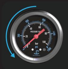
After use, turn the cylinder off and purge the machine by pressing the 'Dual Fire' button, until the gauge returns to the zero pressure.
