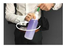
Fill the bottle with your preferred chemical up to the neck of the bottle. Screw the cap into place, being careful not to cross thread
