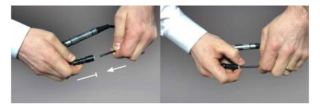
Firstly make sure the connector is facing the right way. The white collar of the connector should point towards the Jet and flow of water. Push the water pipe into the connector until the pipe stops, roughly 7mm. To separate the connection, with two fingers, push the white collar towards the black housing and pull the pipe out.
