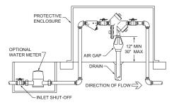
**<u>CAUTION:</u>** Do not pipe the relief valve solidly to a floor drain, sewer or sump.
