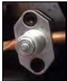
refrigeration line tapping valve
