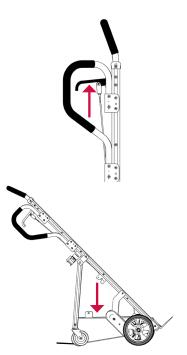
The pivoting center brace must be completely at the end of its travel before the truck can fully support the load!
