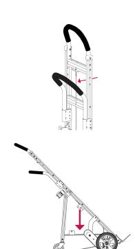
The pivoting center brace must be completely at the end of its travel before the truck can fully support the load!
