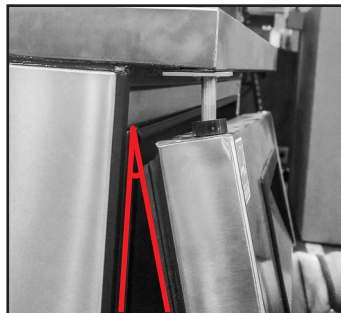
Fig. 10. If needed, only use shallow angles when positioning the door.
