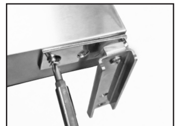
Fig. 5. Remove the cartridge hinge assembly.
