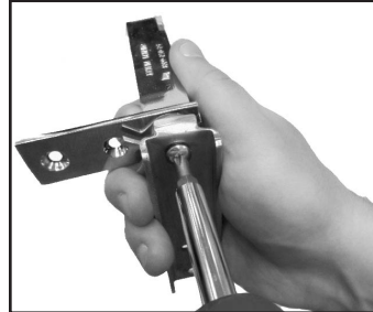
Fig. 6. Remove the hinge bracket from the cartridge spring and then rotate it.
