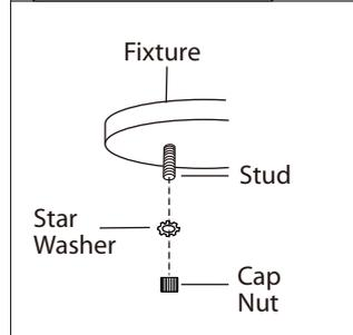
**4.** Tuck electrical wires into electrical box and position fixture over studs on mounting bracket assembly. Secure fixture in place with star washers and cap nuts.
