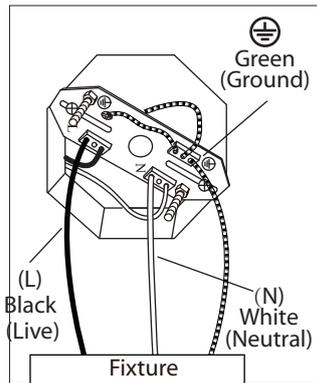
**3.** Connect (push) electrical wires from fixture into correct inserts.
