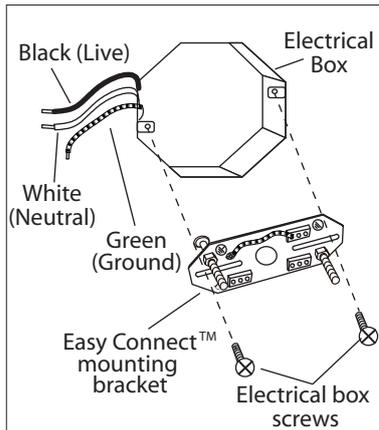
**1.** Attach Easy Connect™ mounting bracket to electrical box with electrical box screws (not included).
