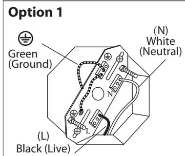
**2. Option 1:** Connect (push) electrical wires from electric box (house wiring) into correct inserts.
