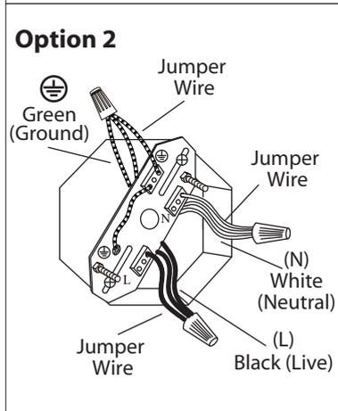
**Option 2:** For multiple green (ground), black (live) and white (neutral) wires joined in the electrical box (house wiring), attach a single “green”, “black” and “white” jumper wire before connecting. Strip 7mm from the 6” jumper wires supplied. Then connect (push) wires into the correct inserts.
