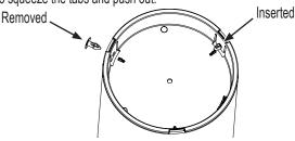
2. Remove the bottom plug, spring, and push plate from the tube.
