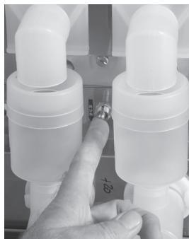
2. Rinse out the Whipper Chambers by placing the RINSE/RUN switch in the RINSE position and activating the DISPENSE switch for 5 to 10 second bursts for each hopper.
