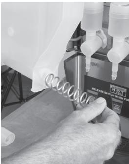
6. Remove the Auger and Auger Drive Shaft by pulling them out the front of the hopper.
