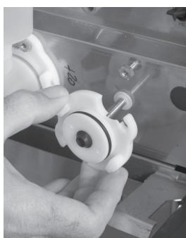
6. Twist Whipper Chamber Receptacle clockwise and pull it off the Motor Shaft.
