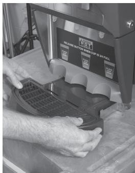
1. Empty the Drip Tray and wash components in a mild solution of dish detergent using a bristle brush. Rinse and dry each item thoroughly before reassembling.
