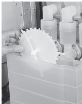
4. Remove the Agitator Disk and Mixing Blades by spreading the hopper walls slightly, and pulling one, then the other Agitator disk shaft end from the hopper wall pivots.
