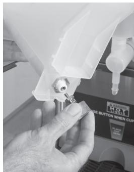
5. Firmly hold Auger with one hand, and remove Auger Drive Coupling by turning it clockwise.
