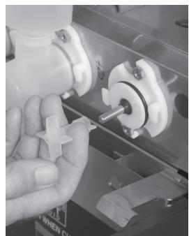
5. Pull the Frother off the Motor Shaft. Notice the flat keyway on the shaft and the matching keyway inside the Frother. It is important that these two keyways are lined up when reassembling.
