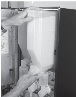
2. Remove the Hopper Assembly from the Cabinet. Remove the Cover and empty the contents.
