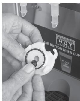
7. Slip the O-ring off the Whipper Chamber Receptacle and remove the shaft seal.
