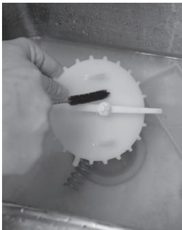
7. Wash all components in a mild solution of dish detergent using a bristle brush when needed. Rinse and dry each item thoroughly before reassembling.
