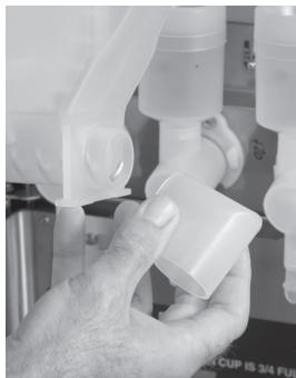
3. Pull the Ejector Elbow off the Hopper Base.
