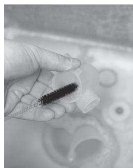
8. Wash components in a mild solution of dish detergent using a bristle brush. Rinse and dry each item thoroughly before reassembling.
